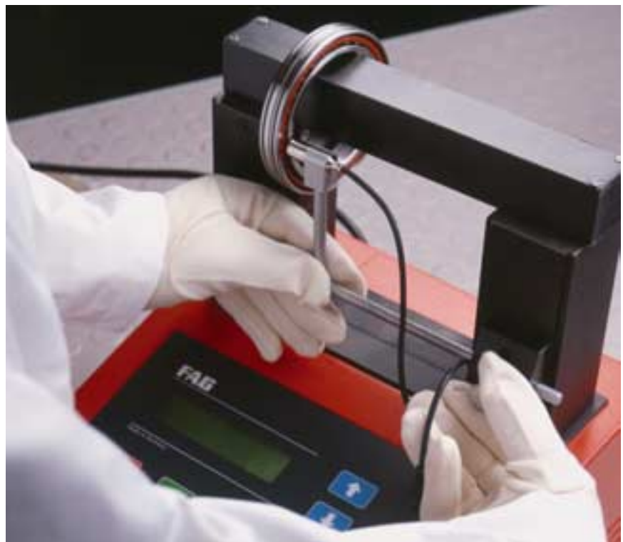
40: Mounting using an induction heating device
